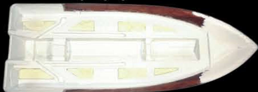
2400 Pure Bay Stringer System with Full Foam Flotation
